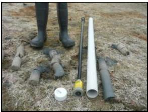
Figure 7. Community developed soil extractor for deeper water monitoring
