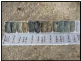
Figure 6. Soil samples in chiptrays.
